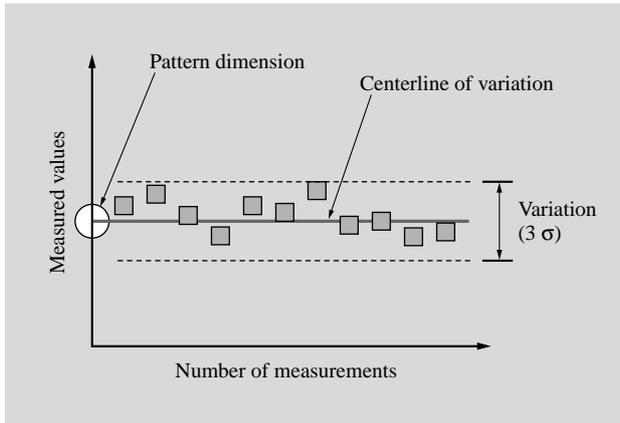
Fig. 5—Example of Measuring Dimension of Pattern without Slimming.
