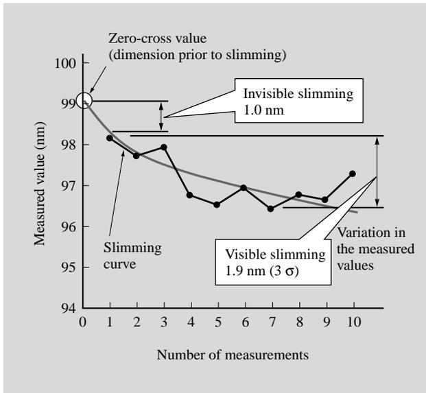
Fig. 4—Reduction of Measured Values Due to Slimming of Resist Pattern.
