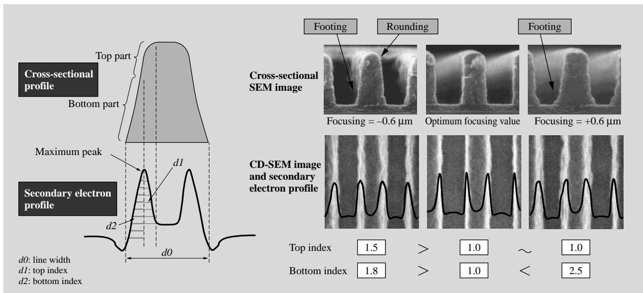
Fig. 10—Focusing Monitor that Uses Top Index and Bottom Index.
