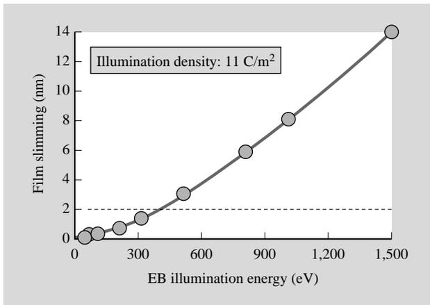
Fig. 8—Example of Slimming Evaluation in Case Where Low- $k$  Film is Illuminated by the EB.
