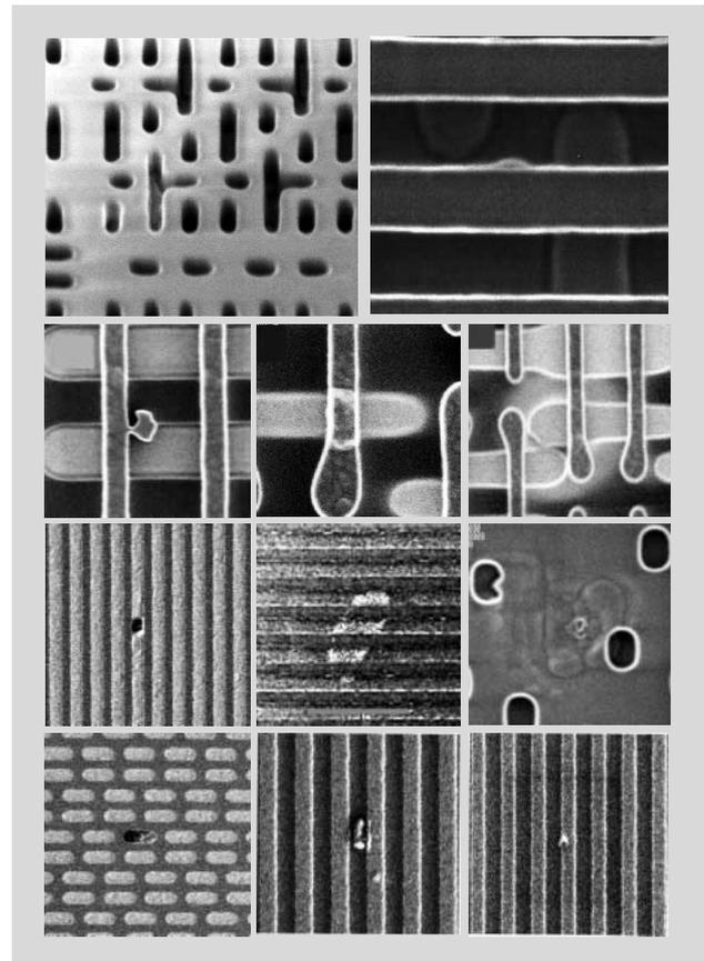
*Fig. 7—Examples of Detected Particles and Defects.*
