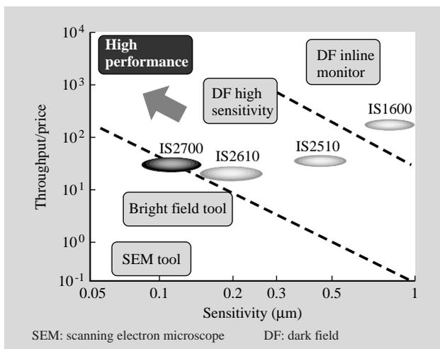
Fig. 2—Throughput/price vs. Sensitivity for IS Series.
