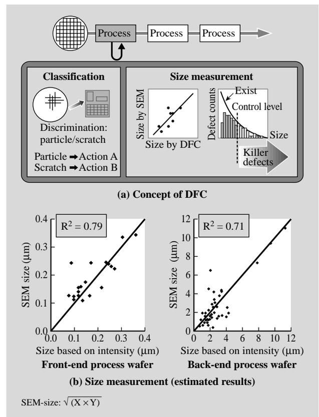
Fig. 4—Defect Classification Function. A DFC function enables defects such as particles and scratches to be classified. The particles sizing function gives an excellent correlation factor of 0.70 between SEM size and standard luminance size.
