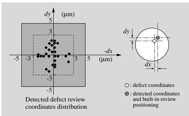
*Fig. 6—Coordinate Accuracy for Linked Analysis Devices.*
