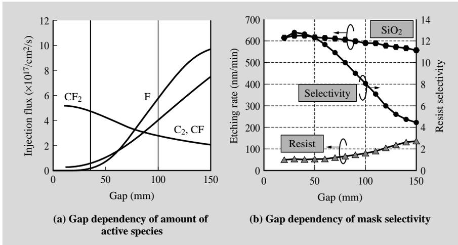
Fig. 4—Control of Active Species in Plasma by Adjusting Gap. For narrow gap settings, mask selectivity is increased. For wide gap settings, good CD control and vertical profiles are obtained.
