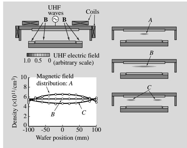
Fig. 3—Principle of Plasma Distribution Control for Etcher. The distribution of plasma is controlled by using coil current to shift where high-density plasma is generated A ← B → C.
