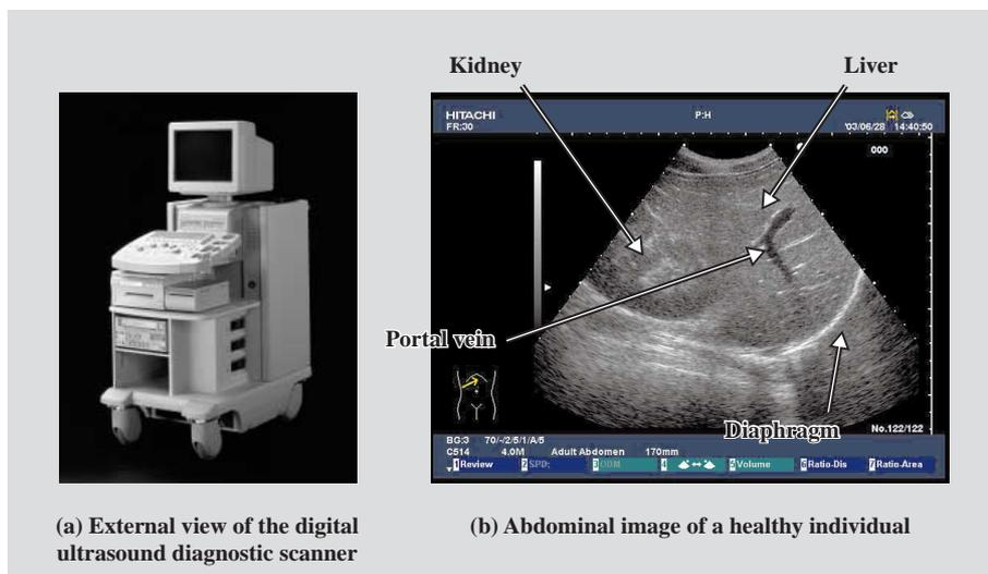
*Fig. 1—External View of Digital Ultrasound Diagnostic Scanner and Abdominal Image of Healthy Individual (right).*
