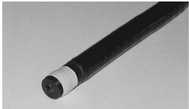
Fig. 10—External View of Electronic Radial Ultrasound Endoscope.
