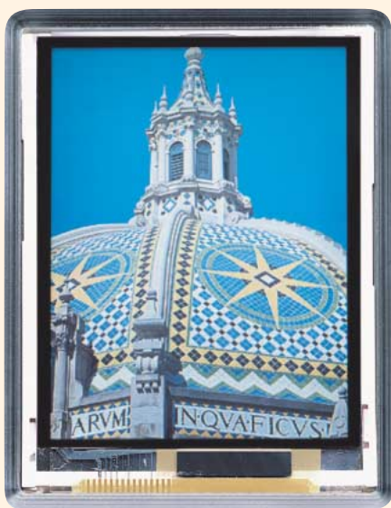
5.6-cm (2.2-inch) QVGA low-temperature poly-Si TFT-LCD
