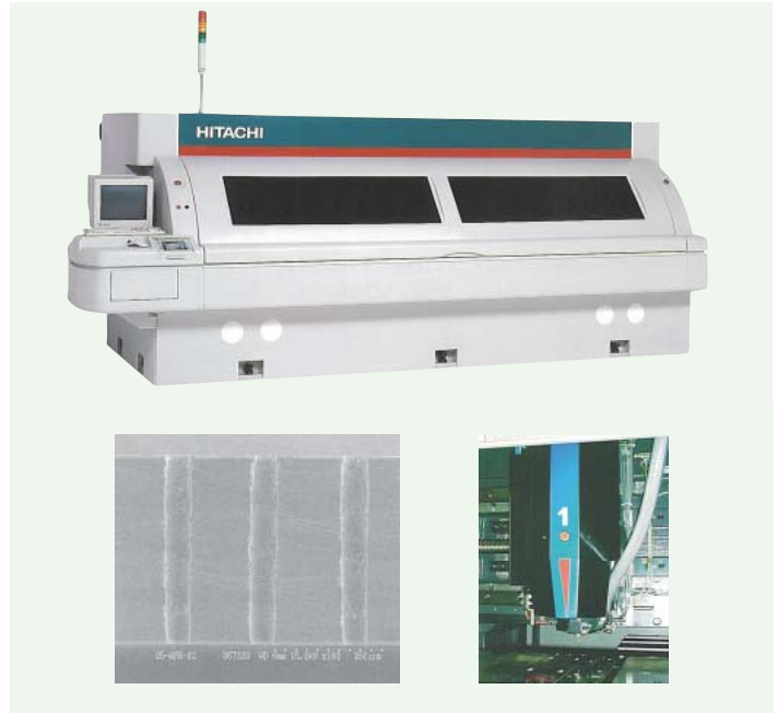
ND-Q series drilling machine with 300,000-min -1 spindles (top), 50-μm via-hole section view (bottom left) and direct-drive z-axis (bottom right)
