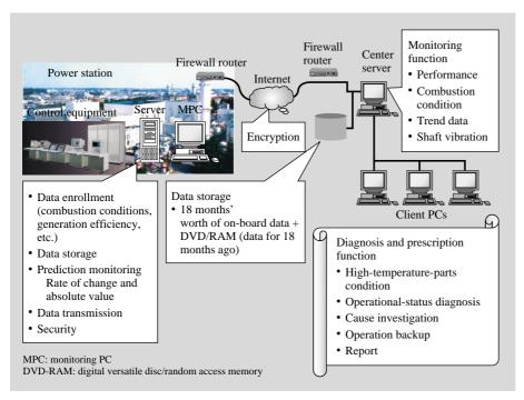
Fig. 5—Overview of Remotemonitoring System.
