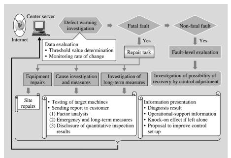
Fig. 6—Process Flow of Monitoring and Diagnosis.
