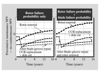
Fig. 3—Example of RBM Evaluation for Maintenance Scenarios Involving Low-pressure Rotor of Aged Steam Turbine. By means of risk assessment for a maintenance scenario, effectiveness of maintenance can be quantitatively evaluated.
