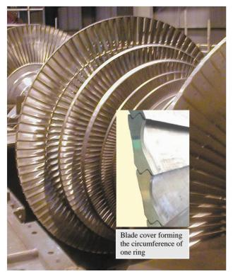
Fig. 4—External View of Low-pressure Rotor Utilizing CCBs for All Blade Stages.
