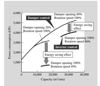
Fig. 1—Power Consumption Reduction Effect with Inverter Control.
