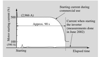
Fig. 5—IDF Starting Current Test Results with Inverter. Compared to commercial operation, motor starting current is reduced by the inverter.
