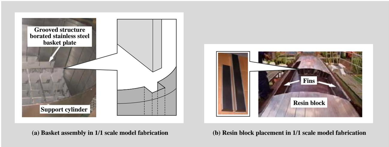
Fig. 4—Outline of Basket Structure (a) and Resin Block Structure (b). To improve reliability and reduce fabrication costs, grooved and block structures were adopted.
