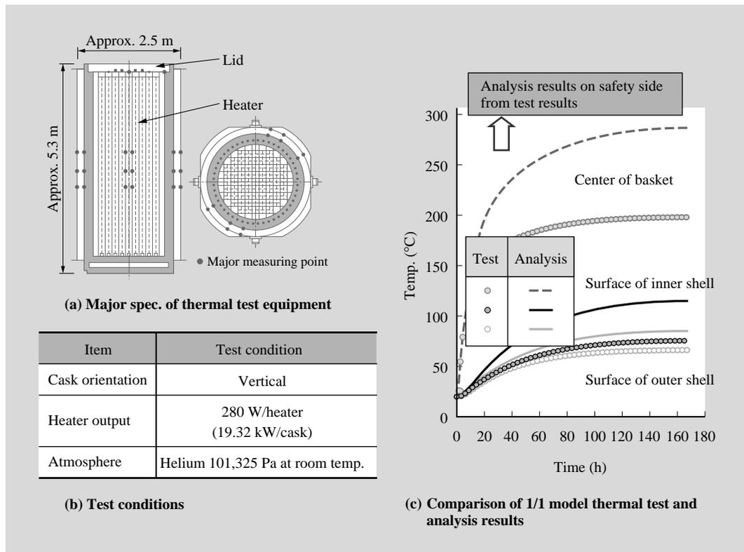
Fig. 8—1/1 Scale-model Thermal Test Conditions and Outline of Results.
