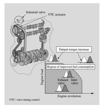
*Fig. 3—Design Features and Structure of Variable-valve-control System.*
