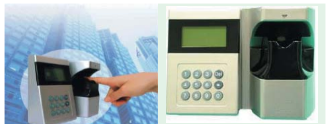
Finger vein scanner detecting the finger vein pattern
