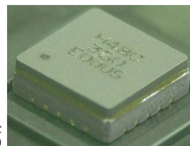
New accelerometer: H48C (4.8 mm 2 × 1.5 mm thick)
