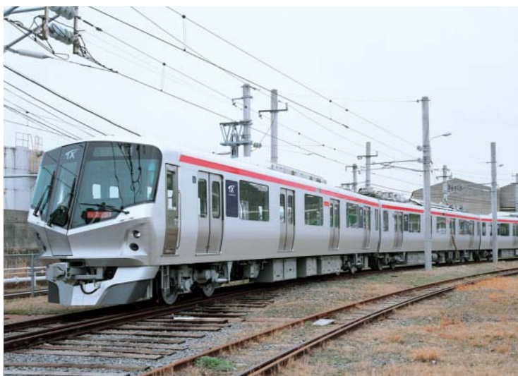
Tsukuba Express dual-voltage AC/DC electric trains
