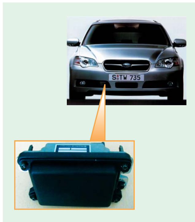
Subaru Legacy Touring Wagon 3.0R with ADA system (above) and Hitachi millimeter-wave radar (below)
