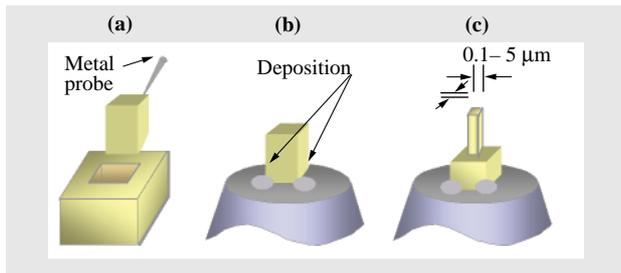
Fig. 3—Micro-pillar Sampling Procedure.
