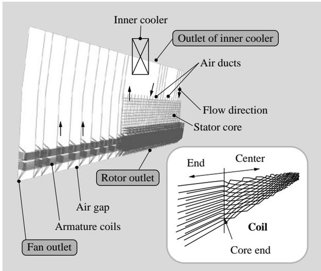
Fig. 3—Schematic of Network for Calculating Stator Temperature. Transposition pitch and wiring arrangement were optimized.
