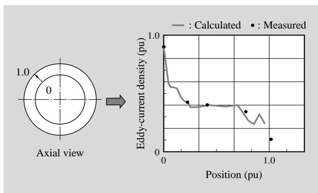
Fig. 8—Example Measurement of Current Density of Copper Shield.
