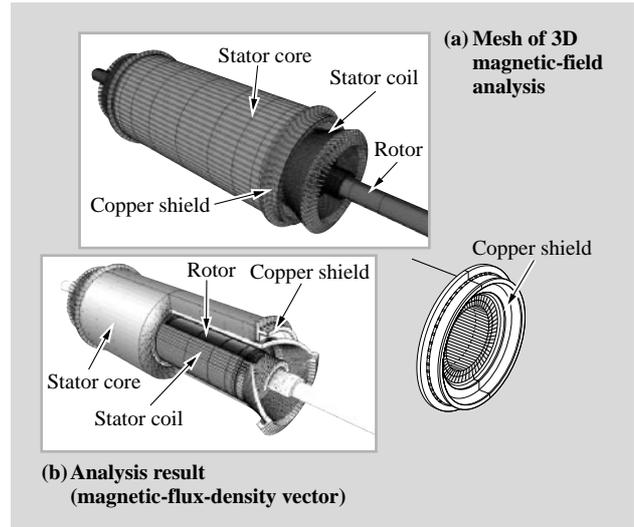
Fig. 4—Example of 3D Magnetic-field Analysis. The stator core structure was optimized according to detailed analysis of magnetic-flux density distribution and loss in the core itself and around it.
