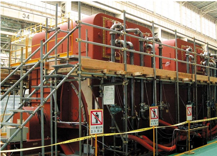
*Fig. 1—Appearance of Performance Evaluation Tests on Generator. Various measurements were performed—namely, on temperature of the strands in the slots of the stator coil, on magnetic-flux density in the stator core and coil end, and current distribution around the core—and the reliability of each part of the generator and the validity of various design tools were confirmed experimentally.*
