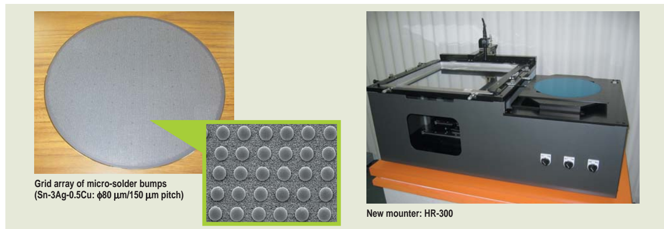
Grid array of micro-solder bumps (left) and new mounter for micro-solder balls: HR-300 (right)
