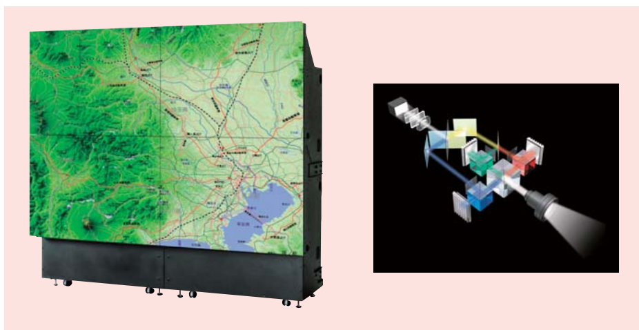
70-inch 2 × 2 LCOS video wall (left) and LCOS optical engine (right)
