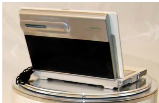
Fig. 9—Example of Mounted Direct Methanol Fuel Cell. External appearance of direct methanol fuel cell mounted on the backside of the display of a laptop PC is shown. As regards refuelling the battery, a cartridge in the top part of the display back face can be simply replaced.
