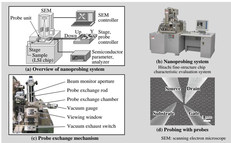
*Fig. 1—Submicron Semiconductor Device Failure Analysis System. While observing semiconductor device patterns with an FE-SEM (field-emission scanning electron microscope), the system uses a nanoprobe with 100-nm tip to evaluate single transistor characteristics and wiring resistances by touching a contact or wiring.*
