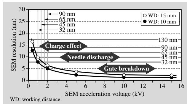
Fig. 3—SEM Resolutions and Acceleration Voltages Required over Next Few Node Generations. Acceleration voltage must be reduced as IC dimensions shrink to enable improved SEM resolution and reduced damage to the chip.
