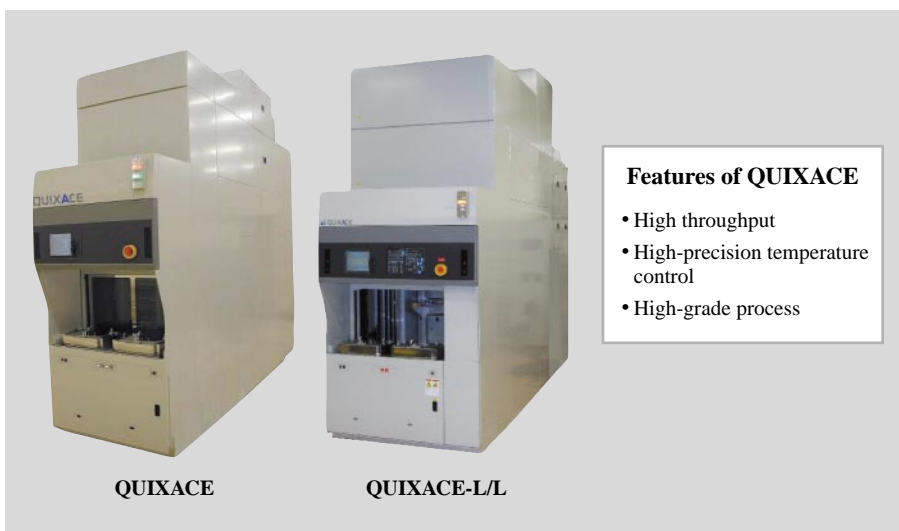
Fig. 1—CVD (chemical vapor deposition)/vertical-diffusion Apparatus “QUIXACE” for Next-generation Devices.
