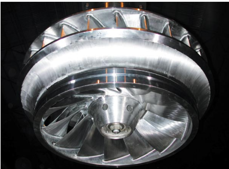
Fig. 1—Water-turbine Runner with Splitter Blades for Otake No. 3 Power Station of THE KANSAI ELECTRIC POWER CO., INC.
