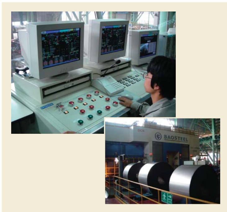
One-person operation in the main control room (above), the mill equipment and cold-rolled coils (below)
