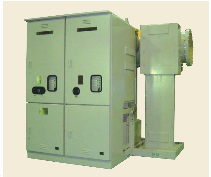
Environmentally friendly GIS (72-kV rated voltage, 800-A rated current, and 25-kA/2-s rated short-time withstand current)
