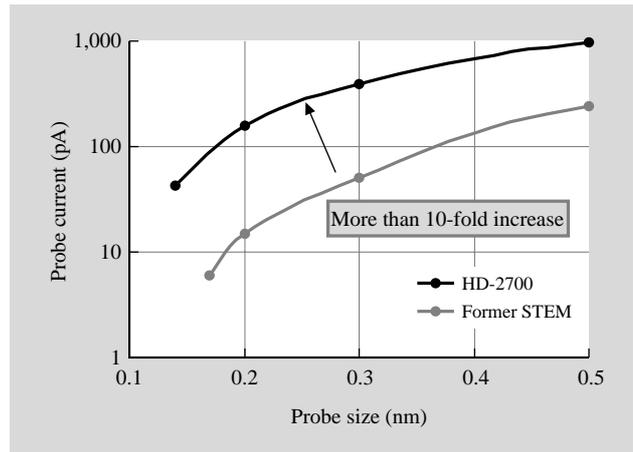
Fig. 5—Probe Size as Function of Probe Current. Probe sizes are estimated; probe current densities are measured.
