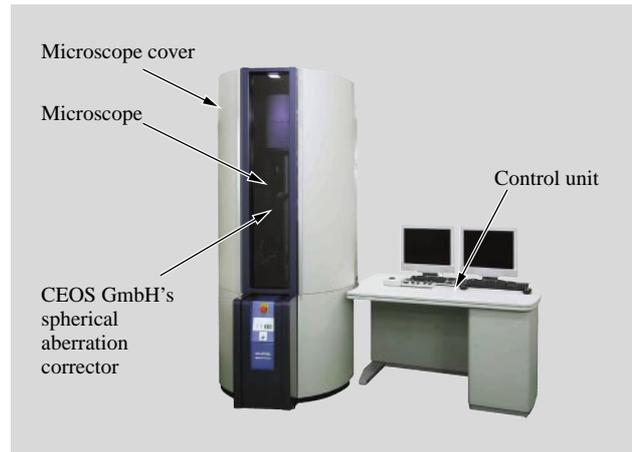
Fig. 3—Photograph of HD-2700. The high-end Cs (objective lens spherical aberration coefficient)-corrected HD-2700 STEM is shown.
