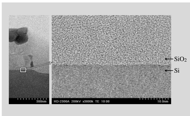
Fig. 7—Bright-field STEM Image of Si Semiconductor Device Cross-section. Capture time is 10 s. The Si crystal lattice and SiO<sub>2</sub> amorphous structure can be clearly observed, indicating that HD-2700 will be a valuable tool for analyzing thicknesses of gate dielectric films.
