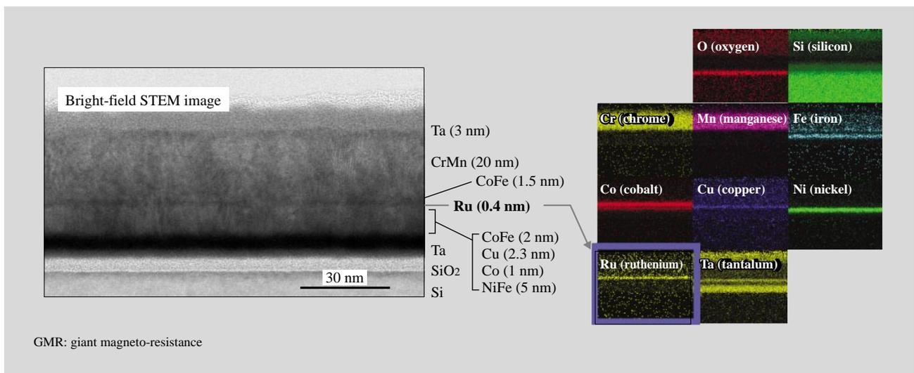
Fig. 9—Bright-field STEM Image of GMR Head Cross-section and EDX Elemental Mapping Image. Probe size is 0.2 nm, probe current density is 150 pA, and capture time is 15 min.
