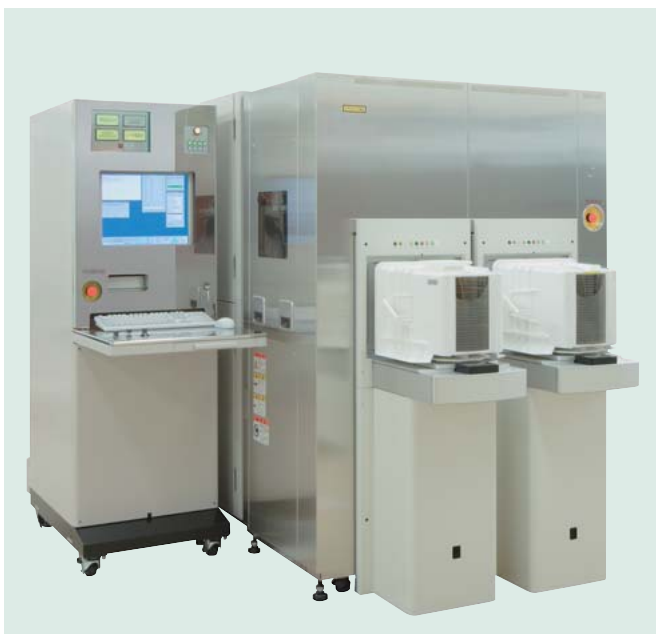
CG4000 high-resolution FEB length meter for next-generation devices
