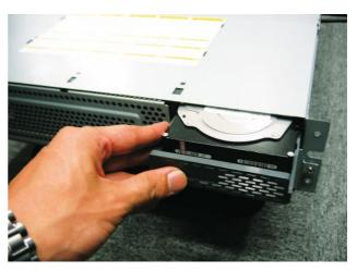
Fig. 4—Inserting an HDD into a Repair Slot.
