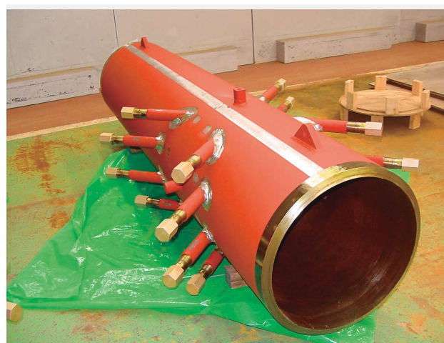
Fig. 5—Chordal Spool for Ultrasonic Feedwater Flow Meter. This spool is girth-welded to the feedwater main pipe. Transducers for transmission and reception of ultrasonic wave are installed on the bosses regularly arranged around the both sides of the spool.
