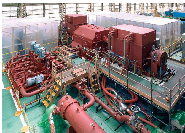
Fig. 7—RIP-MFG System for the Shimane Nuclear Power Station Unit No. 3 of The Chugoku Electric Power Co., Inc. An integrated test was conducted after the actual system was assembled in the factory and connected to the RIP in the RIP test center used for RIP performance testing.
