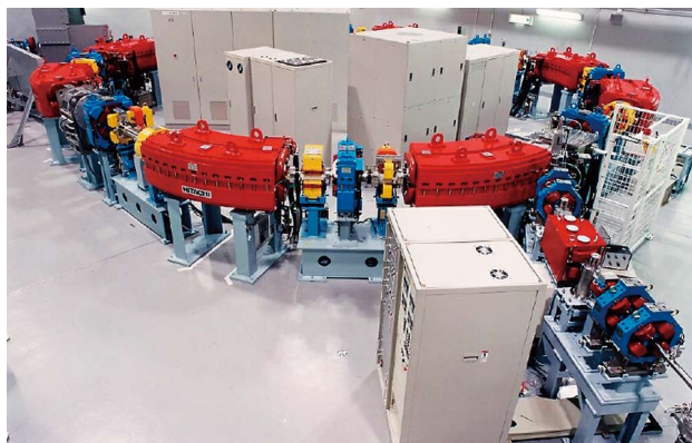
Fig. 5—Wakasa-wan Energy Research Center Multipurpose Accelerator System with Synchrotron and Tandem. Ion beams are widely used in materials science, biology, medical research, and elsewhere [photograph courtesy of the WERC (Fukui Prefecture)].
