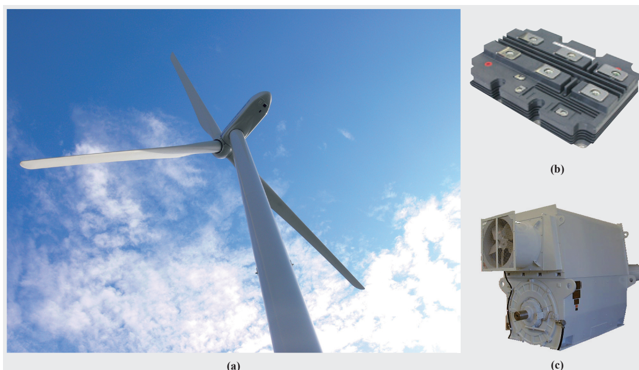
Fig. 1—First SUBARU 80/2.0 2-MW Downwind Turbine to Commence Commercial Production of Electric Power (a), IGBT (b), and Generator (c).
