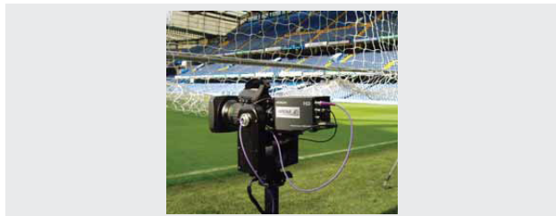
Fig. 9—Example Use of DK-H32 POV (point of view) Camera. Widely used for sports coverage and similar, the DK-H32 supplies dynamic images.
