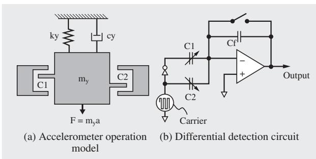
Fig. 10—Accelerometer Detection Principles. Variation in the two differential capacitors ( $C1$ ,  $C2$ ) enables the detection of acceleration (in both  $x$  and  $y$  axes).
