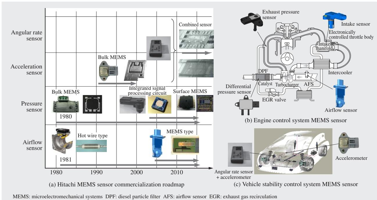
Fig. 1—Hitachi MEMS Sensor Roadmap and Positions of Various Sensors in Vehicle. The history of Hitachi's development of sensors applying MEMS technology, as well as the positions of on-board sensors used for automobile control are shown. The development and adoption of MEMS technology has expanded the range of applications for automobile sensors.
