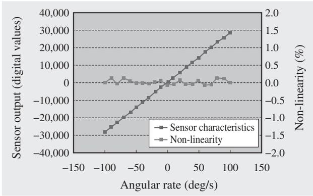
Fig. 9—Angular Rate Sensor Characteristics. The non-linearity of the angular rate sensor output characteristics is  $\pm 0.2\%$  F.S. (full scale) or less.
