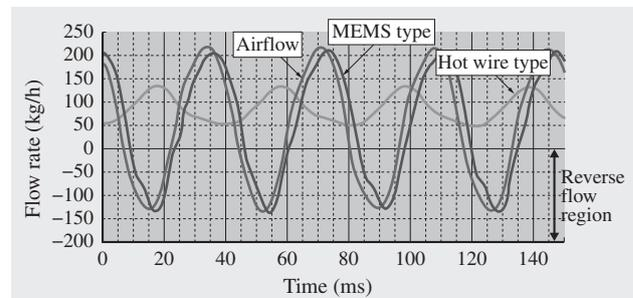
Fig. 4—Hot Wire and MEMS Sensor Flow Characteristics. The MEMS sensor's characteristics with respect to airflow allow for the accurate measurement of flow rate in the reverse flow region as well.
