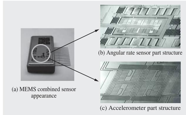
Fig. 7—MEMS Combined Sensor. The angular rate and acceleration elements are each formed on the silicon substrate and mounted in a single package.
