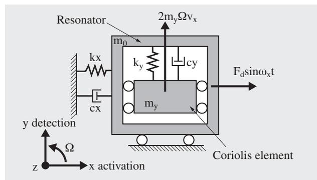
Fig. 8—Angular Rate Sensor Detection Principles. When the resonator vibrates in the direction of the  $x$  axis and an angular rate is applied around the  $z$  axis, the Coriolis element is displaced in the direction of the  $y$  axis.
