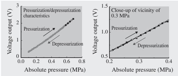
Fig. 6—MEMS Pressure Sensor Characteristics. Measurements without hysteresis are realized within a range of 0.1 to 1 MPa.
