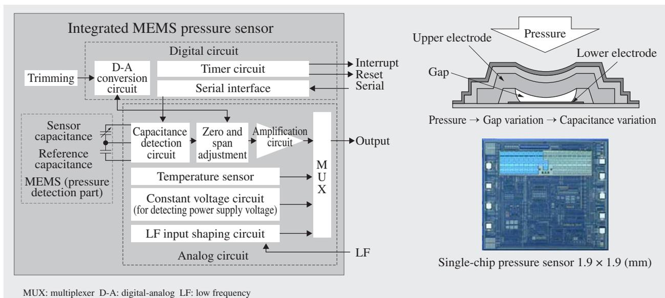
Fig. 5—MEMS Pressure Sensor Principle, Chip Configuration, and Appearance. The MEMS element and circuit are integrated into a single chip.
