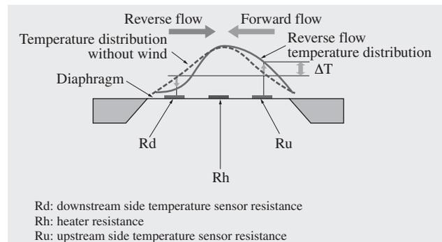
Fig. 3—MEMS Airflow Sensor Detection Principle. The placement of detection elements formed on a diaphragm enables the measurement of forward and reverse flows.
