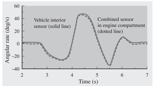
Fig. 12—Combined Sensor Cold Region Testing with Actual Vehicles. The angular rates from the vehicle interior sensor and the combined sensor are synchronized, making it possible to accurately measure vehicle behavior.
