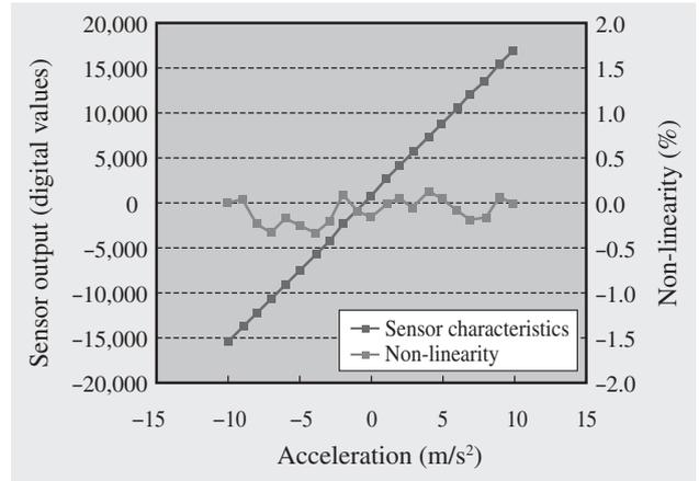
Fig. 11—Accelerometer Characteristics. The non-linearity of the accelerometer output characteristics is  $\pm 0.4\%$  F.S. or less.
