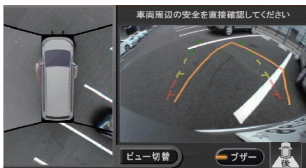
Fig. 4—Example Display from Around-view Monitor. The monitor simultaneously displays the composite bird's eye view next to the conventional front or rear display.
