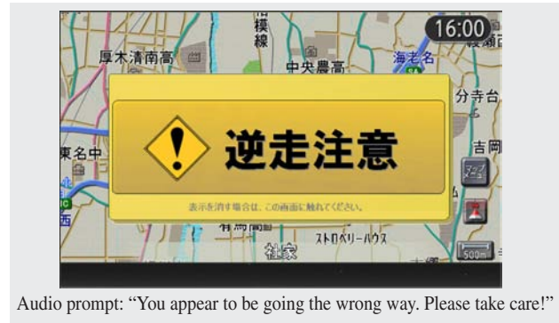
Fig. 7—Example Screen from Wrong-way Warning System. Both audible and on-screen warnings are issued.
