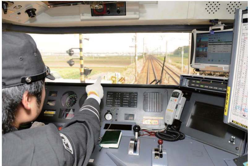
Display terminal in operating train (top right of the photograph) (photograph courtesy of Japan Freight Railway Company)
