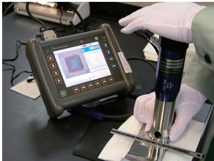
Testing for plastic strain (hardness measurement)
