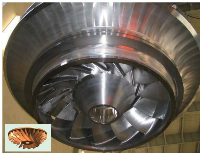
Splitter blade runner for Shinnakachiyama Power Plant of Hokuriku Electric Power Company and three-dimensional CAD (computer-aided design) drawing (lower left)
