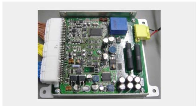
Fig. 7—Integrated Battery Controller for Hybrid Vehicle Battery System.
