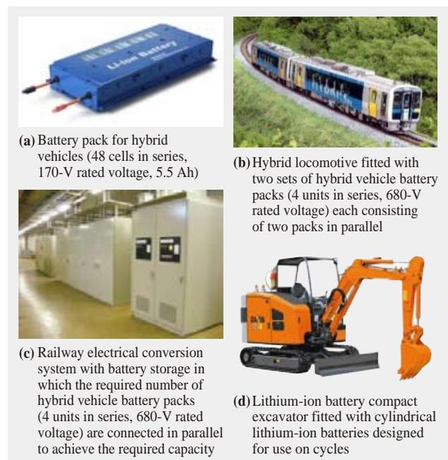
Fig. 9—Industrial Applications of Lithium-ion Batteries. Examples of industrial applications for Hitachi lithium-ion batteries are found in various industries.
