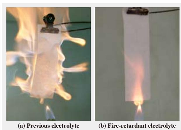
Fig. 4—Electrolyte Flammability Test. By equipping the electrolyte with self-extinguishing properties, the fire risk was largely eliminated.
