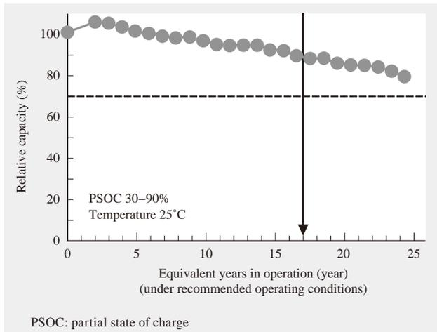
Fig. 3—Results of Battery Life Testing of New LL-W Battery. The batteries achieved a life equivalent to more than 17 years of operation under recommended operating conditions.
