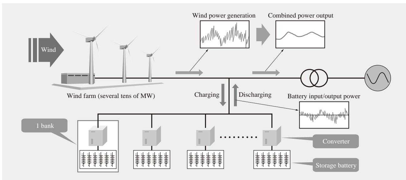
Fig. 1—Overview of Use of Storage Batteries at Generation Sites to Stabilize Output Fluctuation. The variation in system output can be stabilized by charging and discharging batteries.
