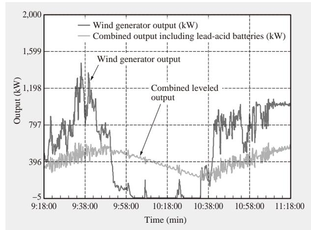
Fig. 2—Example of Output Leveling at Wind Power Generation System Incorporating Storage Batteries. The graph shows how variation in the system output can be stabilized by charging and discharging batteries.
