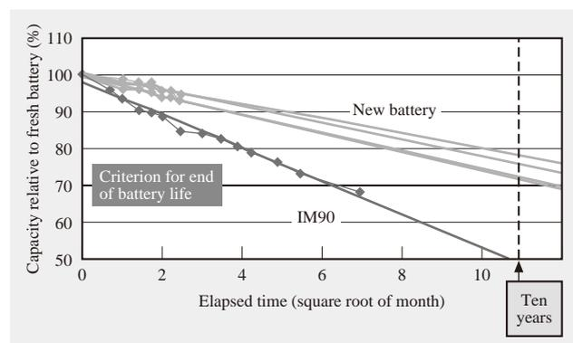
Fig. 5—Change in Battery Capacity with Age under Float-charge Conditions.
