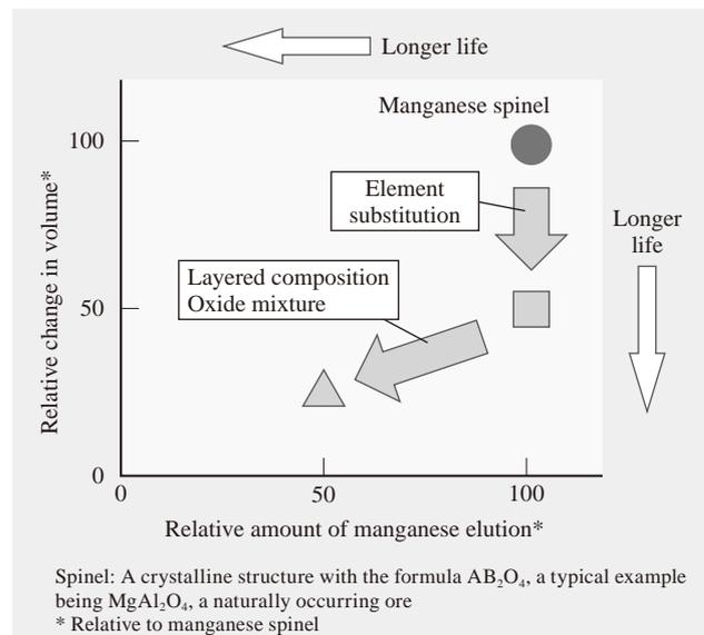
*Fig. 3—Extending Life of Manganese-based Cathodes. The crystal structure of the cathode was stabilized by substituting some of the manganese in the manganese spinel with different elements and elution of manganese was suppressed by mixing in layered composite oxides with excellent acid-resistance. The result of these improvements is a projected battery life of ten years or more.*
