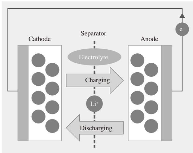
*Fig. 2—Principle of Operation of Lithium-ion Battery. A lithium-ion battery works by releasing electrons through the transfer of lithium ions between cathode and anode electrodes that sandwich a separator impregnated with electrolyte. The cathode and anode are made of materials that are able to intercalate and deintercalate lithium ions respectively.*
