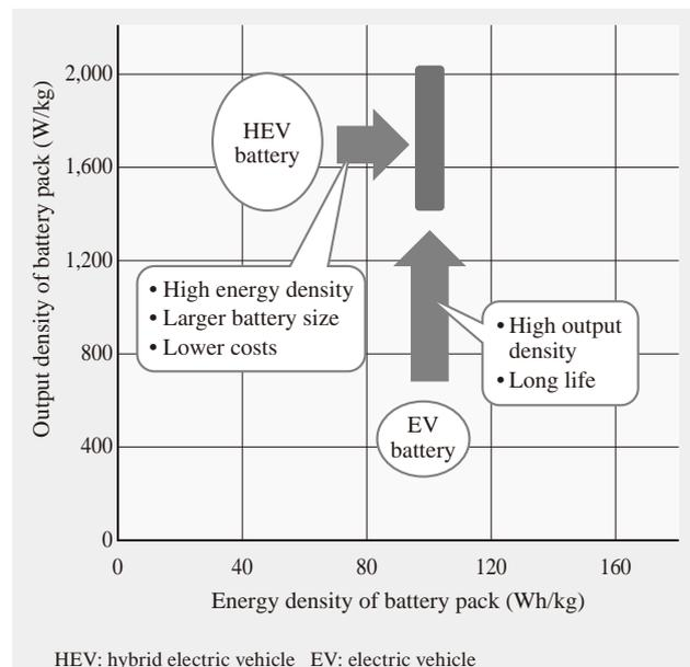
Fig. 1—Characteristics Required in Large Lithium-ion Batteries.
