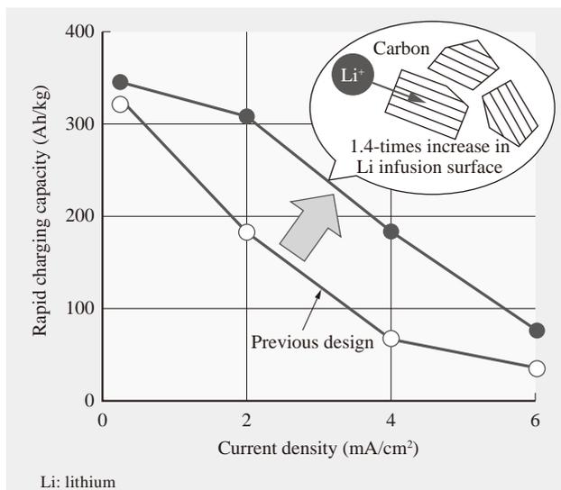
Fig. 4—Rapid Charging Capacity of Carbon Anode. Improvements to heat treatment, grinding, and other production processes succeeded in enlarging the area of infusion surface through which lithium ions are intercalated and deintercalated by 1.4 times. This significantly enhanced the rapid charging characteristics.
