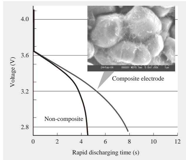
Fig. 6—Rapid Discharging Performance of Composite Electrode.
