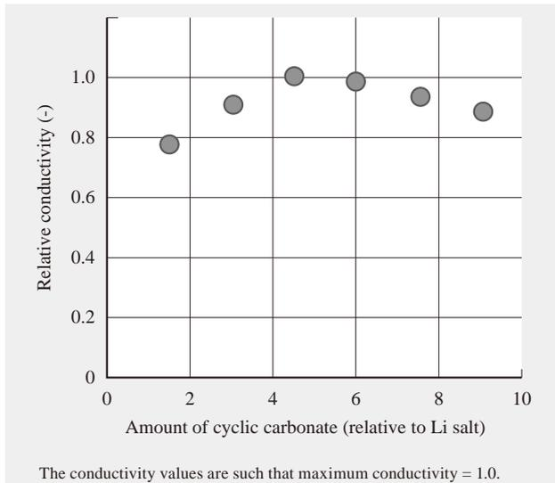
Fig. 5—Effect of Cyclic Carbonate Content on Electrolyte Conductivity.
