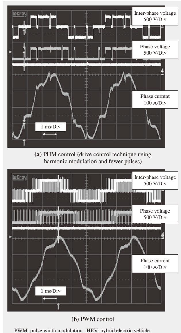
Fig. 8—PHM Control (Elimination of 5th Harmonic) and PWM Control (10-kHz Carrier).
