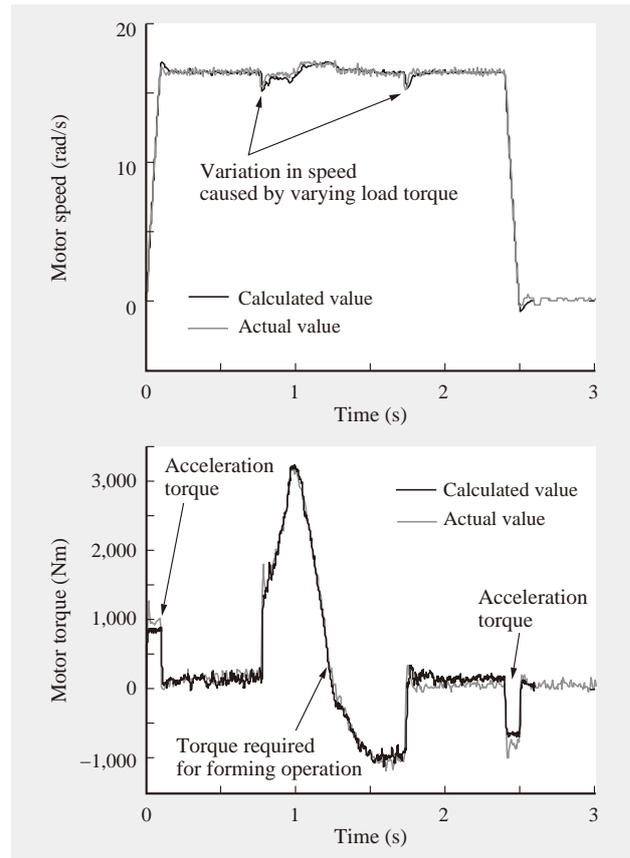
Fig. 10—Example Calculation Using Integrated Simulator.
