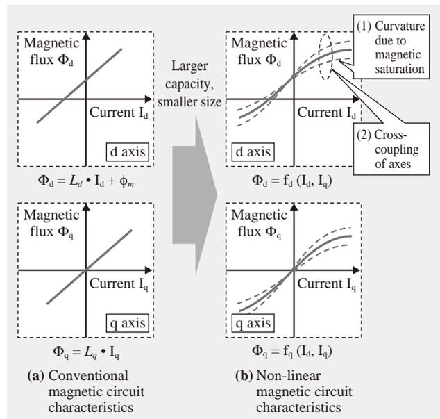
Fig. 5—Magnetic Circuit Non-linearity of Flux in Motor. The relationship between current and magnetic flux is a curve (non-linear) rather than a straight line (linear), and cross-coupling also occurs between the  $d$  and  $q$  axes.
