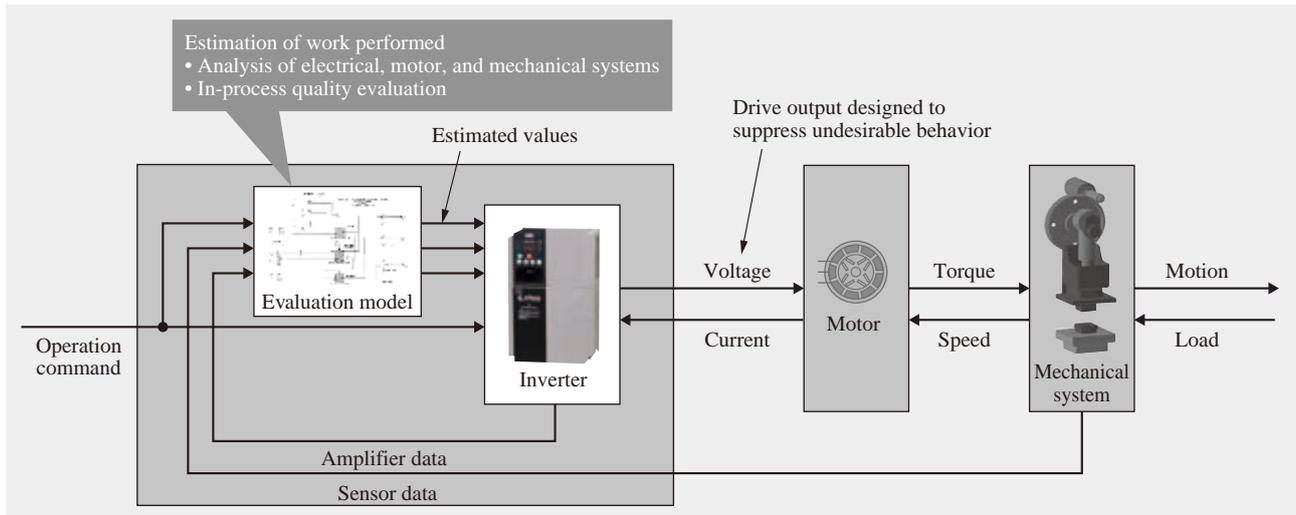
Fig. 11—Use of Evaluation Model of Mechanical System to Enhance Control Performance.
