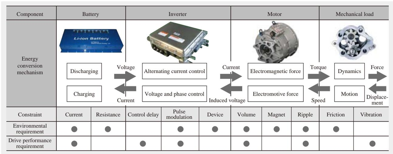
Fig. 2—Interrelationships between Components in Electric Drive Applications. Harmonious control of the electric drive system is achieved by considering the interrelationships between the battery, inverter, motor, and mechanical load based on their respective energy conversion mechanisms.
