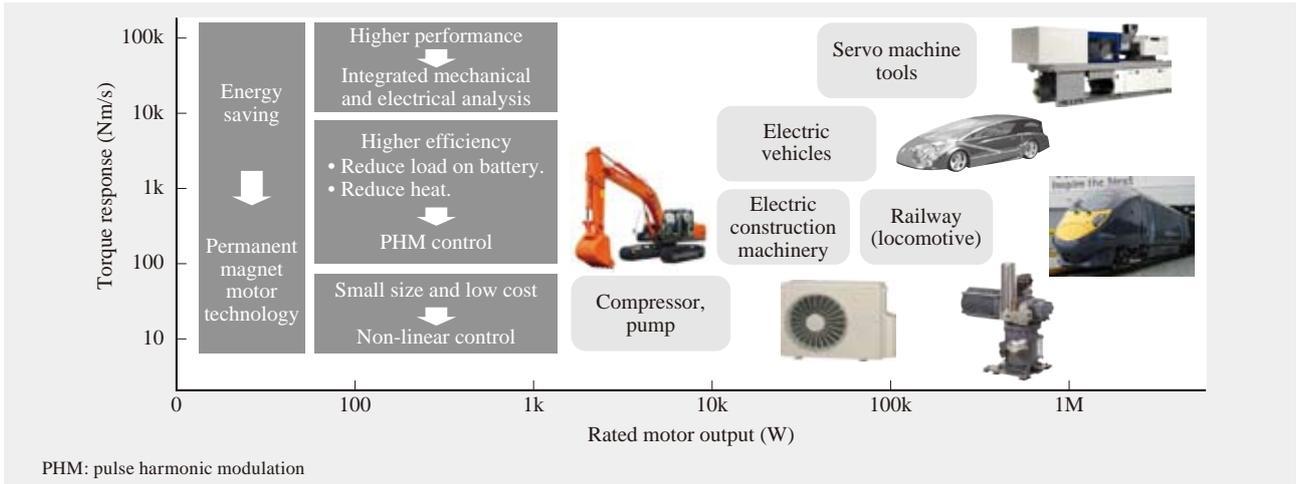
Fig. 3—Core Technologies for Electric Drive Systems. These systems are based on electric drive of a permanent magnet motor and feature new control techniques and effective analysis techniques for system design.
