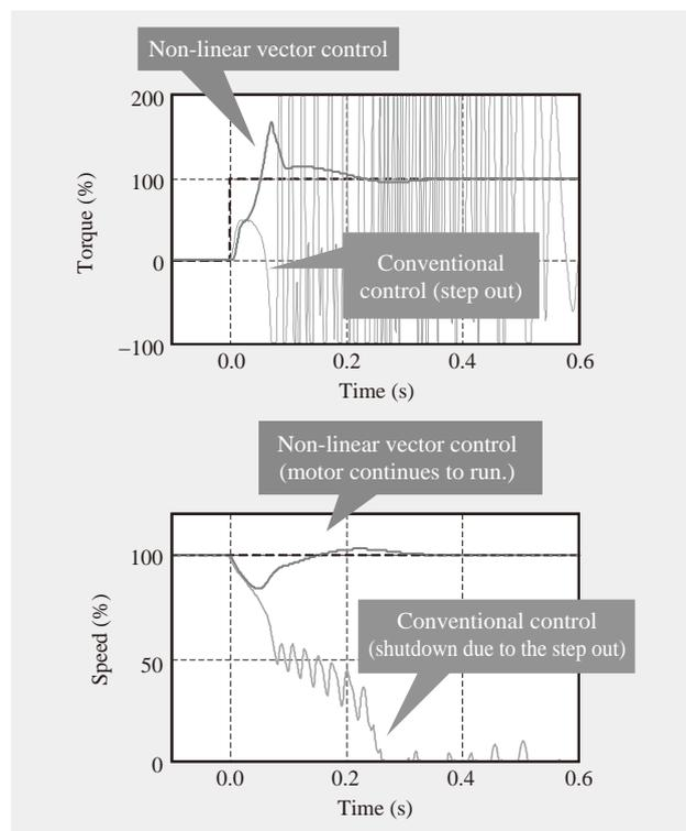
Fig. 7—Comparison of Responses to the Out-of-range External Impact Load by Motor with Highly Non-linear Characteristics (Simulation).
