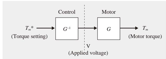
Fig. 4—Relationship between Motor Characteristics and Control. Flexible motor torque control can be achieved by implementing a control system based on an inverse model of the motor’s transfer function ( $G$ ).
