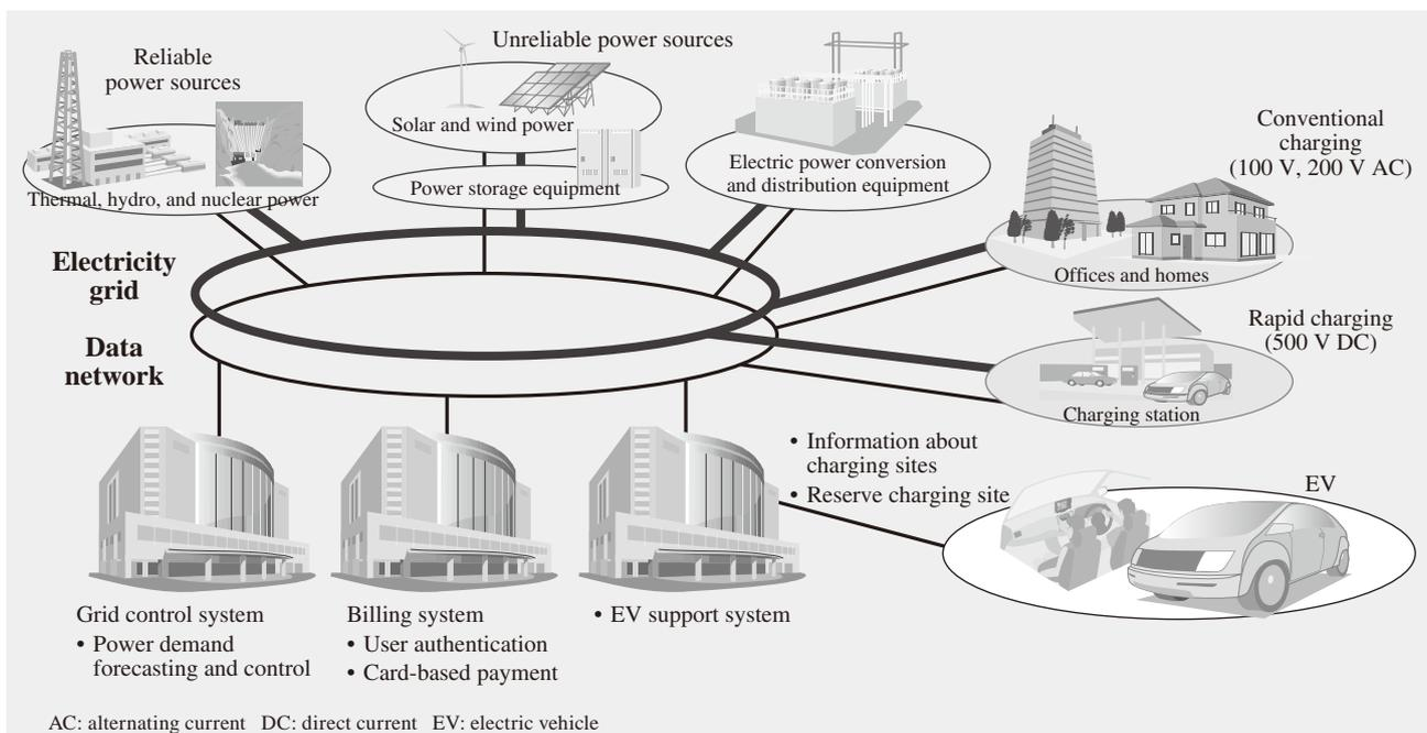
Fig. 4—Concept of Driving Support and Charging Systems for EVs. The EVs, charging systems, and driving support work together to form a smart grid.
