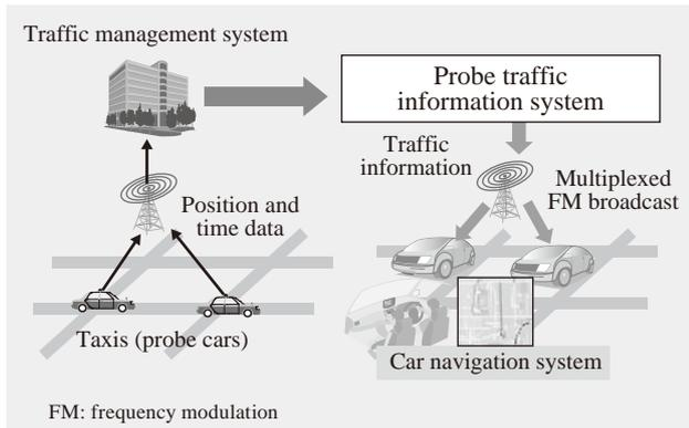
Fig. 3—Overview of Probe Traffic Information System in Beijing. Traffic information is generated from position data collected from 2,000 taxis and used to provide details of traffic congestion to the car navigation systems in the demonstration vehicles.
