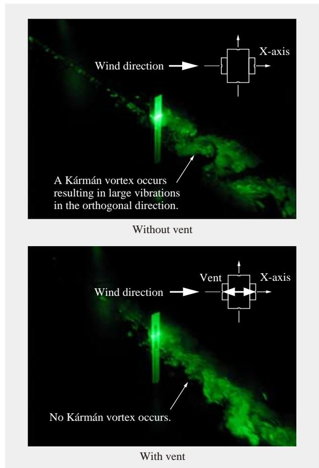
Fig. 5—Wind Tunnel Testing.
