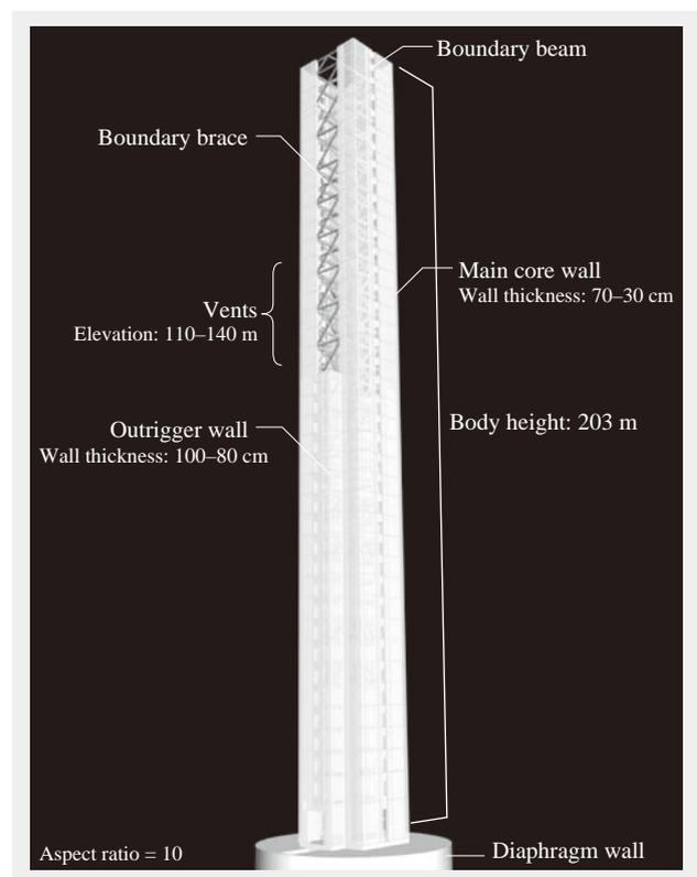
Fig. 2—Perspective Drawing of Tower Structure. The tower body has a height of 203 m and the total height is 213.5 m.
