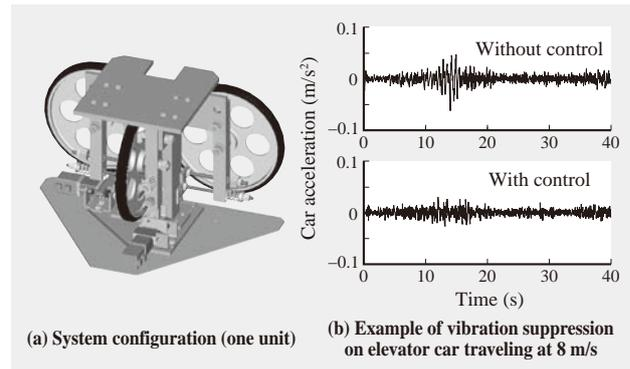
Fig. 8—Configuration and Effects of Active Guide Unit.
