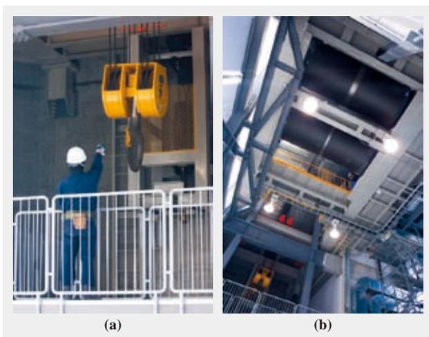
Fig. 6—Large-capacity Winch. The winch has a lifting height of 210 m. Photograph (a) is a front view of the hook and photograph (b) is a view of the traction machine seen from below.
