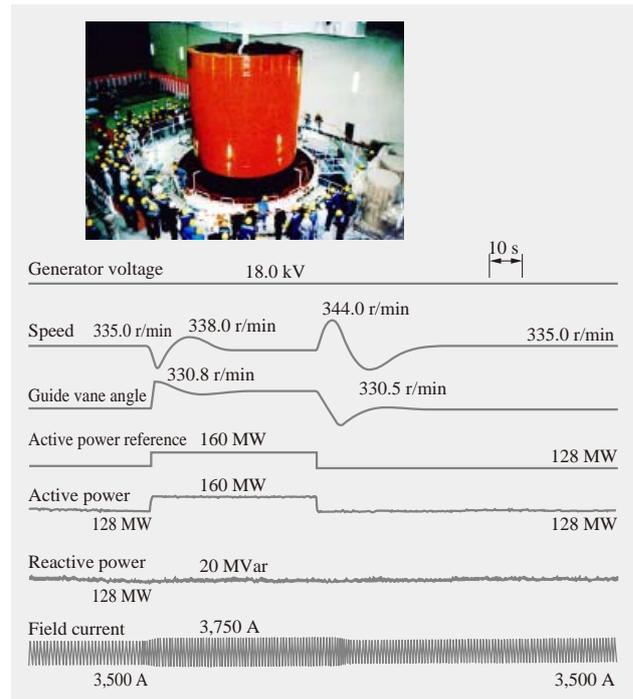
Fig. 2—Adjustable-speed Pumped-storage Generation System Supplied to Okawachi Power Plant of The Kansai Electric Power Co., Inc.
