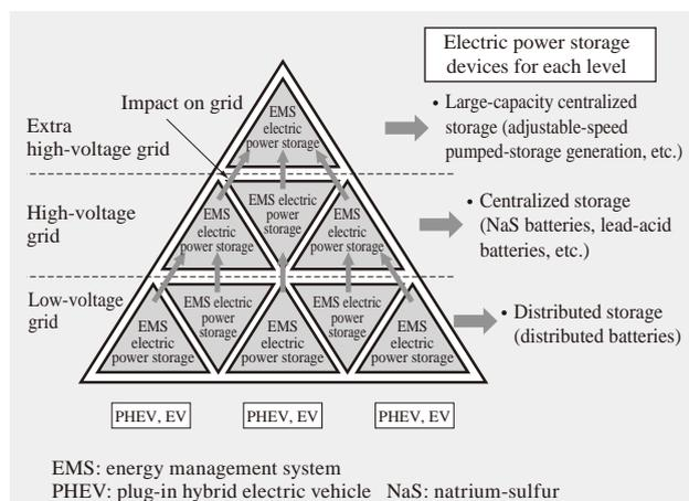
Fig. 5—Concept of Electric Power Storage for Future Grid. The concept is to maintain stability and power quality for the entire grid by utilizing storage batteries to localize the influence of photovoltaic power and EVs within each demand cell.
