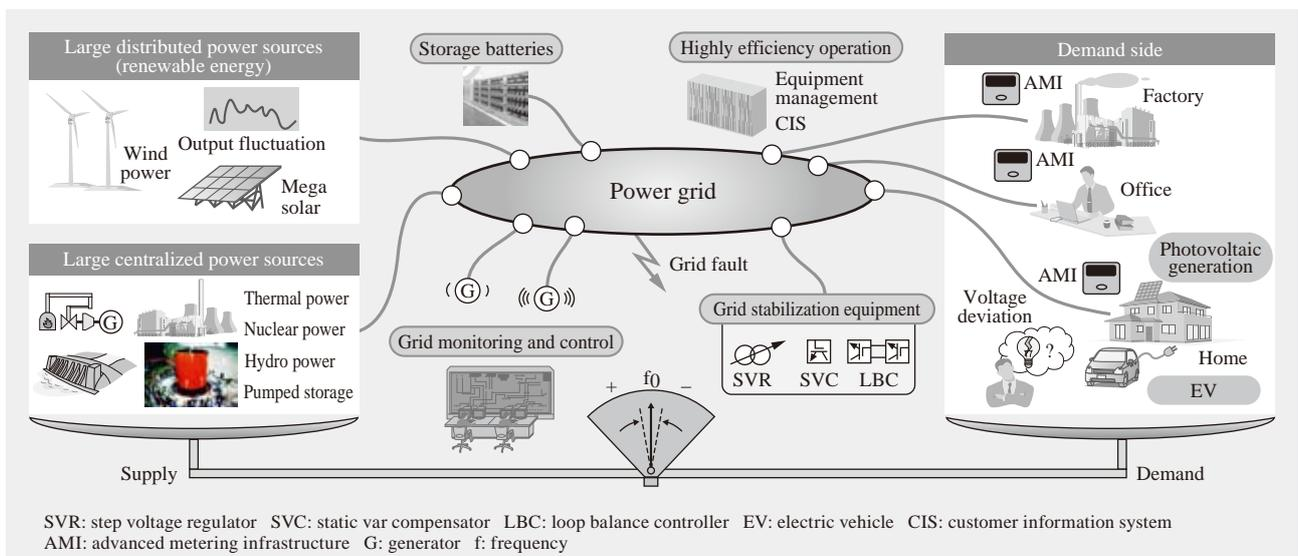
Fig. 1—Overview of Next Generation of Power Grid Systems.
