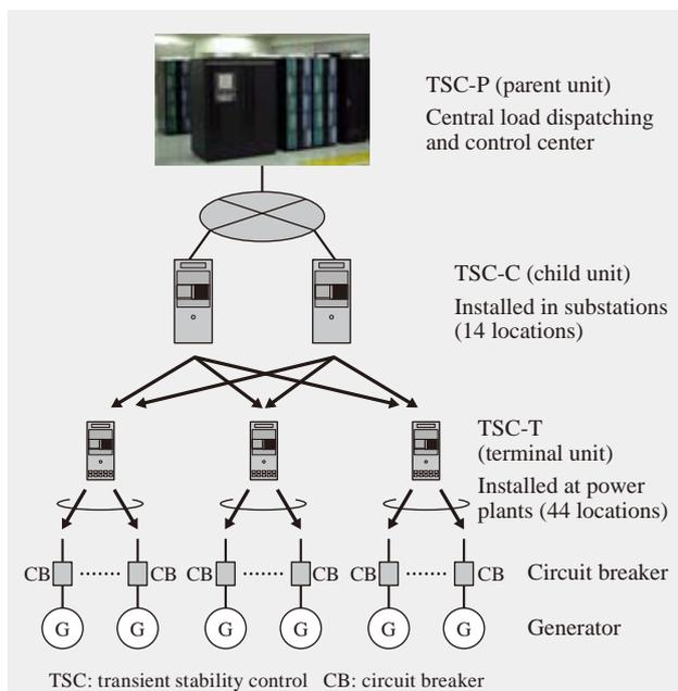
Fig. 3—Online Transient Stability Control System Supplied to Chubu Electric Power Co., Inc.
