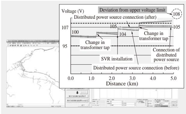
Fig. 7—Overview of High-voltage Analysis System for Distributed Power Sources.
