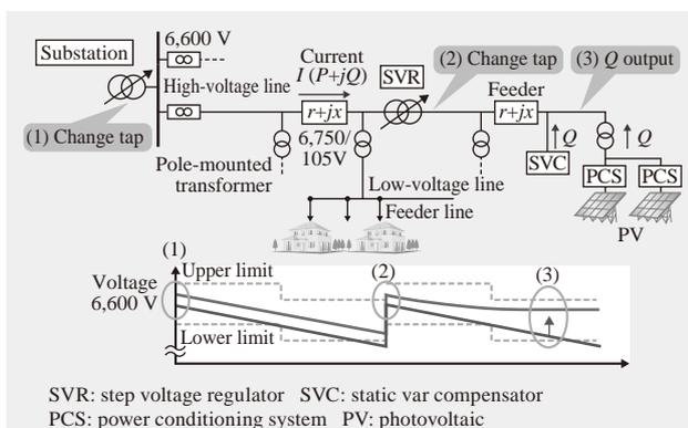
Fig. 1—Overview of Grid Voltage Control.
