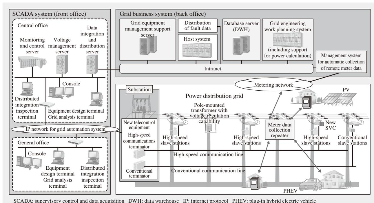
Fig. 2—Example Configuration of SCADA System.
