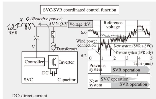
Fig. 3—Self-commutated SVC for Use on Grid (300 kVA). The system can coordinate operation with an SVR using local data.
