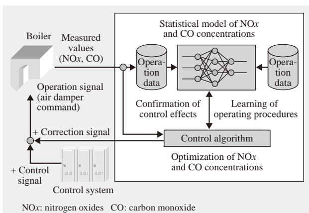
Fig. 3—Configuration of Control System for Reducing Environmental Impact. Self-tuning control with reinforcement learning provides corrective values which optimize the concentrations of NO<sub>x</sub> and CO.
