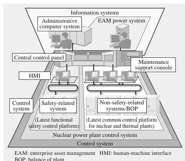
Fig. 4—Concept behind Control System for New Nuclear Power Plants. This figure shows an overview of an information and control system for smart NPPs.
