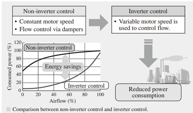
Fig. 2—Energy Savings Achieved by Inverter Control. Using inverters for flow control in place of damper systems reduces power consumption.
