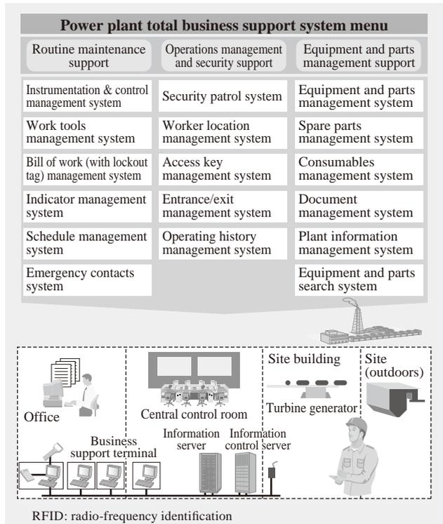
Fig. 8—Periodic Inspections Assistant System Using RFID. This integrated business support system for daily plant operation uses RFID technology.
