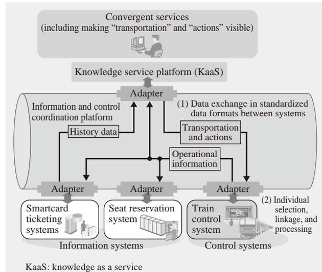
Fig. 3—Convergence of Information Systems and Control Systems in System Architecture for Services.
