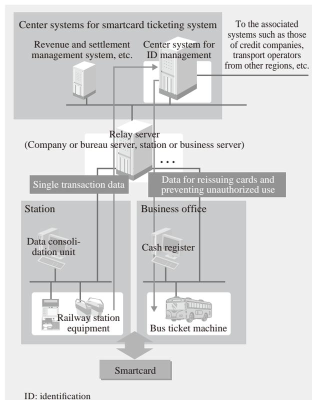
Fig. 3—Overview of Smartcard Ticketing System. Data on smartcard use (itemized transaction data) is sent from terminals to the center system and the accumulated data used for reissuing cards and preventing unauthorized use.
