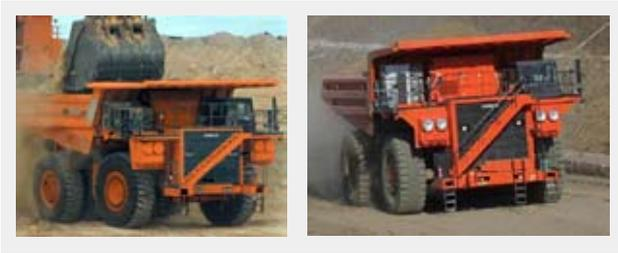
Fig. 9—EH3500ACII and EH4000ACII. These dump trucks use an AC-IGBT (alternating current—insulated gate bipolar transistor) electric drive system jointly developed by Hitachi Construction Machinery Co., Ltd. and Hitachi, Ltd.
