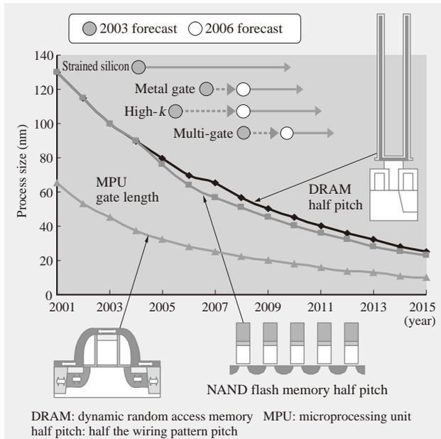
Fig. 3—Microfabrication Technology Forecast in International Technology Roadmap for Semiconductors (ITRS).
