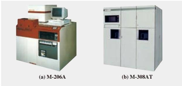
Fig. 2—Equipment Developed through Special Research Program. A beta tool incorporating a magneto-microwave plasma source was installed at the Device Development Center in late 1984. After design improvements and process evaluation, the unit was re-installed as the first upgraded M-206A in late 1985 (a). The M-308AT was introduced to the market in 1987. Based on the M-206A, it also incorporated further upgrades and an on-board post-etch processing module (b).
