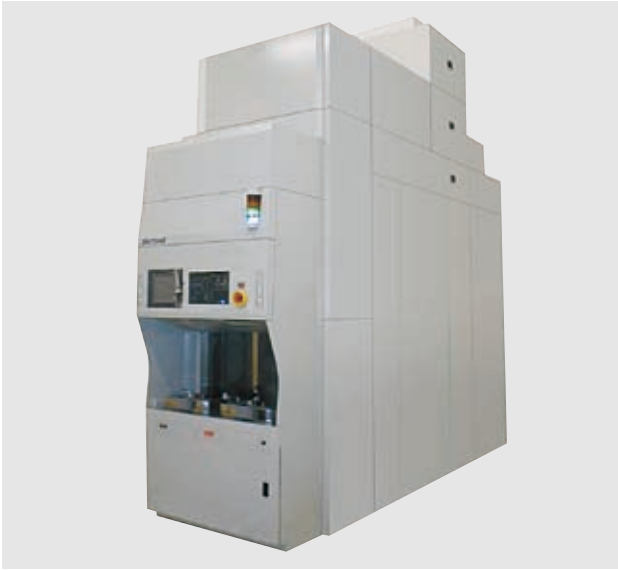
Fig. 3—QUIXACE Vertical Annealing Furnace for 300-mm Wafers. The furnace supports applications ranging from temperatures as low as 150°C up to a very high 1,350°C.
