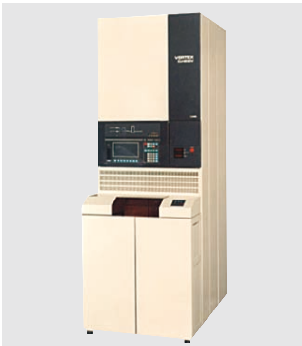
Fig. 1—First Vertical Furnace. Hitachi, Ltd. and Hitachi Kokusai Electric jointly won a technology award from The Japan Society of Mechanical Engineers in 1992 for their success in developing vertical heater technology.
