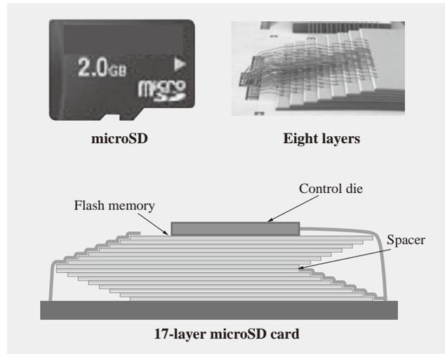
Fig. 3—External View and Interior Structure of Memory Card. A photograph of a microSD card, a SEM (scanning electron microscope) image of its interior (eight layers), and a diagram of its structure (17 layers) are shown. Bonding a large number of identical dies together in a single package allows higher memory capacities to be achieved.
