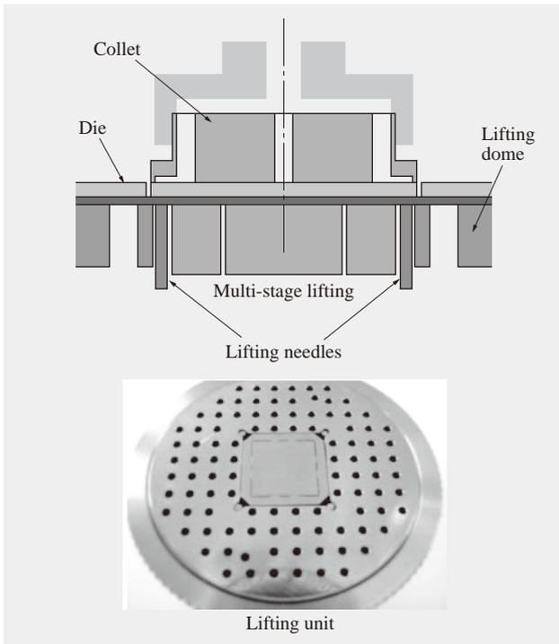
Fig. 2—New Lifting Mechanism. The lifting mechanism allows thin dies to be layered. A feature of the mechanism is that it minimizes stress due to bending of the die.
