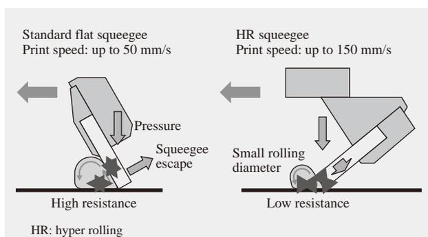
Fig. 8—Overview of Squeegee Operation. Using HR squeegee can reduce the contact resistance with the solder during rolling and achieve high coverage even under high-speed printing conditions.
