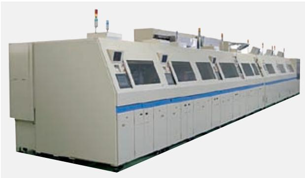
Fig. 7—AL/AB7000 Module Assembly System. This module assembly system for the production of wide panels up to 57 inches in size is an integrated line able to perform all steps from driver IC to PCB mounting.
