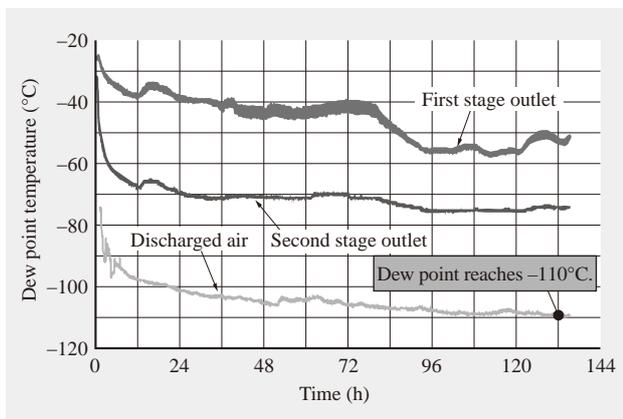
Fig. 11—Change in Air Dew Point Temperature over Time. The graph shows operating data for the super clean ultra-low dew-point air generator system at startup. The results demonstrate the excellent dehumidification performance of the system, with the dew point of the discharged air reaching  $-100^{\circ}\text{C}$  after 20 hours and  $-110^{\circ}\text{C}$  after 6 days.
