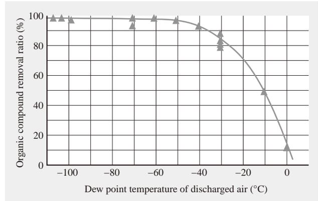
Fig. 12—Relationship between Dew Point Temperature and Organic Compound Removal Performance. The performance at removing organic compounds improves as the dew point falls, reaching better than 99% removal when the dew point is below  $-100^{\circ}\text{C}$ .
