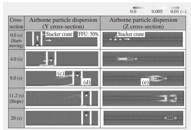
Fig. 4—Analysis Results for Airflow and Airborne Particle Dispersion when Local Ventilation Used to Improve Cleanliness. The extent of airborne particle dispersion in the cassette stocker is reduced by the use of local ventilation.
