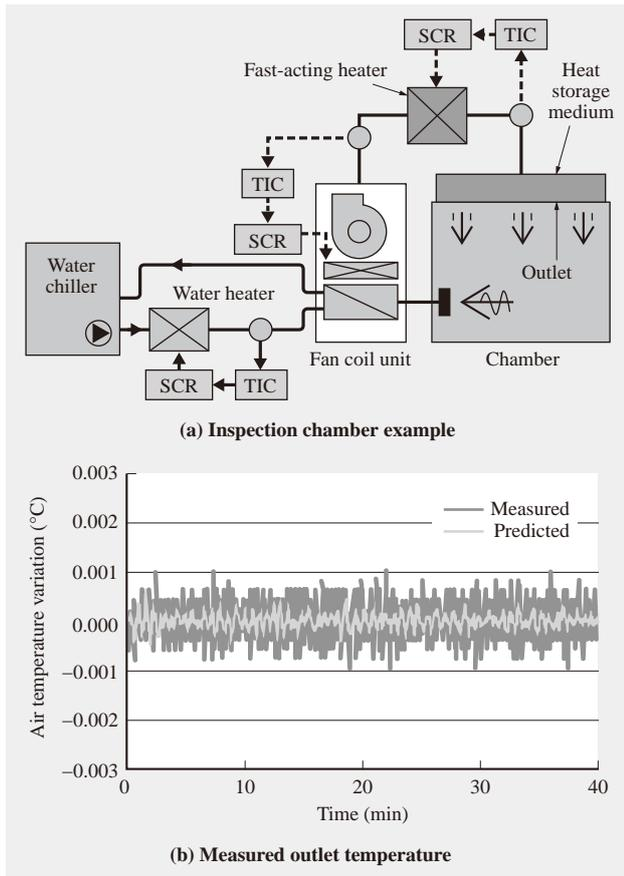
Fig. 7—Application of Air Conditioning System with Precise Temperature Control in Inspection Chamber. The system was installed in a semiconductor component inspection chamber where it demonstrated its ability to control the outlet temperature in the  $\pm 0.001^{\circ}\text{C}$  range.
