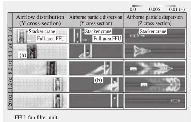
Fig. 3—Analysis Results for Airflow and Airborne Particle Dispersion in Cassette Stocker when Stacker Crane in Motion. The analysis indicates how operation of the cassette stocker causes the dispersion of airborne particles inside the stocker chamber. This is due to the airflow and airborne particle dispersion that occur when the stacker crane lifts a cassette while in motion.
