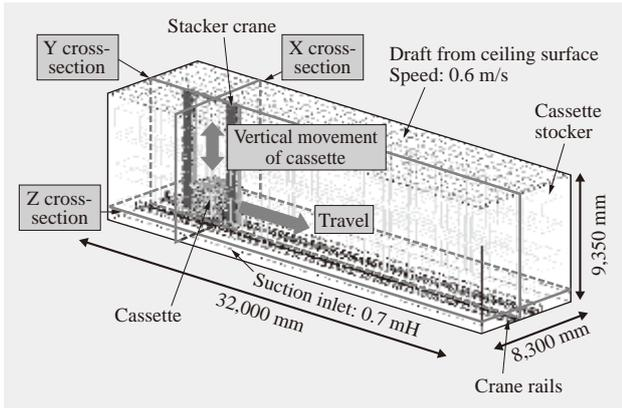
Fig. 2—Cassette Stocker Model. An overview of the model used to analyze a cassette stocker used for temporary storage of LCD (liquid crystal display) substrates.
