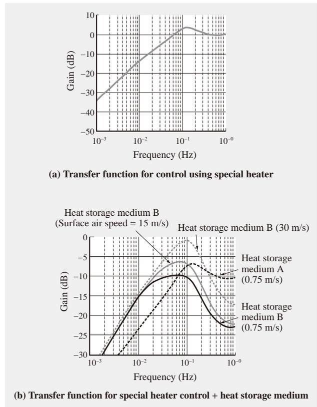
Fig. 6—Transfer Function for Special Heater and Heat Storage Medium Combination.
