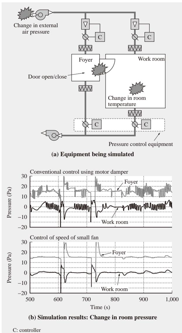
Fig. 9—Performance Comparison of Pressure Control Equipment Using Pressure Control Simulation. A comparison was made of the performance of two different types of pressure control equipment in response to external influences (variations in external air, door opening and closing).
