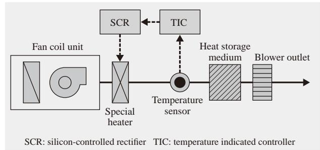
Fig. 5—Air Conditioning System with Precise Temperature Control. Characteristics include a quick-acting heater, minimization of temperature fluctuations through use of heat storage medium, and other techniques.
