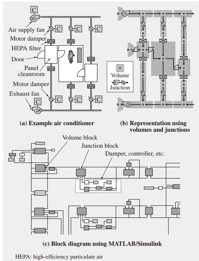
Fig. 8—Overview of Pressure Control Simulation for Air Conditioner.
