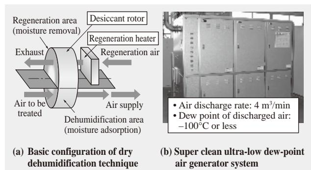
Fig. 10—Principles of Super Clean Ultra-low Dew-point Air Generator Technology and Equipment Photograph. The system works on the principle of dry dehumidification and consists of three desiccant rotors connected in series.
