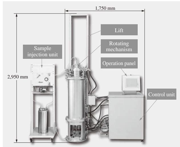
Fig. 5—Hitachi CC40NX Continuous Flow Ultracentrifuge. First released in October 2009, the ultracentrifuge has a maximum speed of  $40,000 \text{ min}^{-1}$  and numerous features including support for steam sterilization of the sample flow path and electronic recording of operating data.
