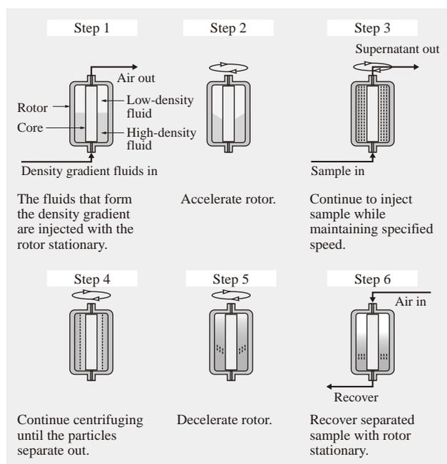
Fig. 4—Operating Procedure for Continuous Flow Centrifugation. Continuous flow centrifugation forms a density gradient in the fluid inside the rotor. This causes the target material to separate out in the density gradient band from which it can be recovered.
