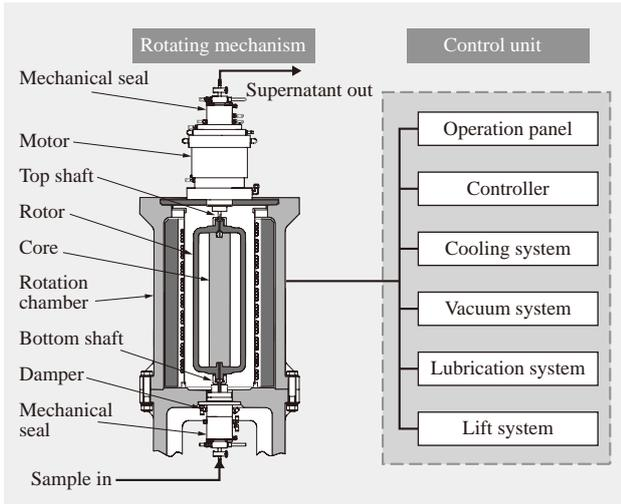
Fig. 2—Structure of Rotating Mechanism and Control Unit. The centrifuge is driven by a high-frequency motor. The sample is introduced via the bottom mechanical seal, separation takes place inside the rotor, and then the supernatant (leftover material) is discharged from the top mechanical seal.
