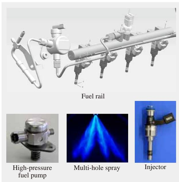
Fig. 5—Fuel Supply System for Direct Injection Engines. These components are used in the fuel supply sub-system for direct injection engines.
