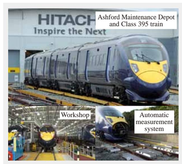
Fig. 4—Ashford Maintenance Depot for Class 395. The photographs show parts of the maintenance depot for the 29 Class 395 trains which operate on conventional track in Kent in the southeastern UK and also the High Speed 1 (HS1). The workshop has five service tracks and the ability to install and remove under-floor components. Outside, the depot has automatic measurement systems that can automatically perform train wheel, brake pad, and other measurements.
