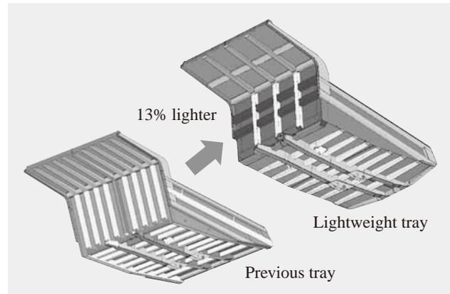
Fig. 2—Reducing Weight of Dump Truck Tray. A redesign of the structure using a strength evaluation technique succeeded in reducing the tray weight by 13% compared to the previous design.
