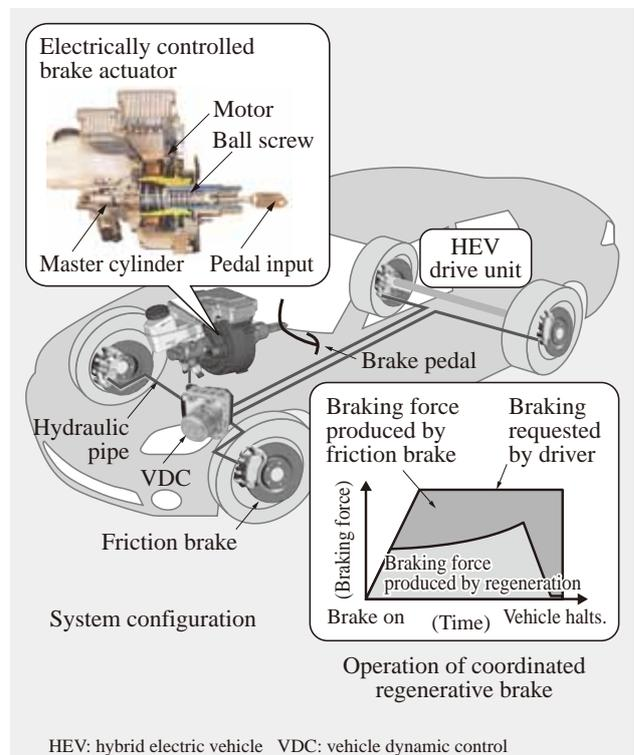
Fig. 6—Electrically Controlled Brake System Supplied to Nissan Motor Co., Ltd. The diagram shows the location and design of the brake actuator together with an example of how the friction and regenerative braking forces are balanced based on how hard the driver is applying the brake pedal.
