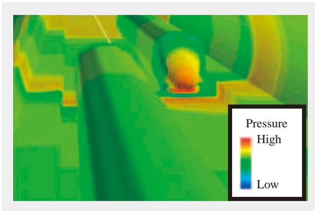
Fig. 3—Distribution of Pressure on Tunnel and Train Walls as Trains Pass through Tunnel.
