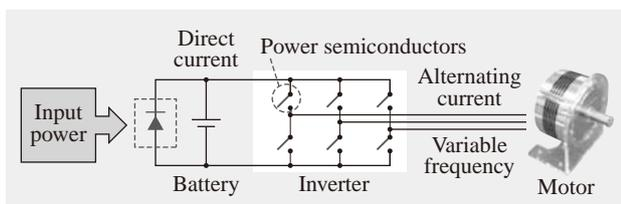
Fig. 1—Configuration of Electric Drive System Using Power Electronics.
