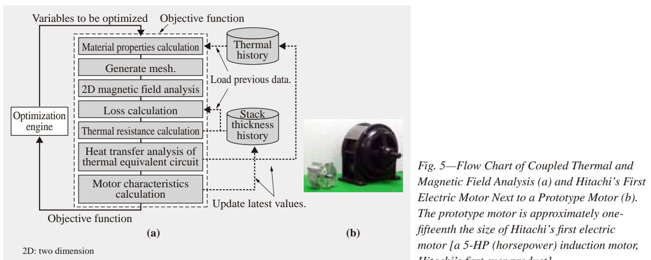
Fig. 5—Flow Chart of Coupled Thermal and Magnetic Field Analysis (a) and Hitachi's First Electric Motor Next to a Prototype Motor (b). The prototype motor is approximately one-fifteenth the size of Hitachi's first electric motor [a 5-HP (horsepower) induction motor, Hitachi's first ever product].
