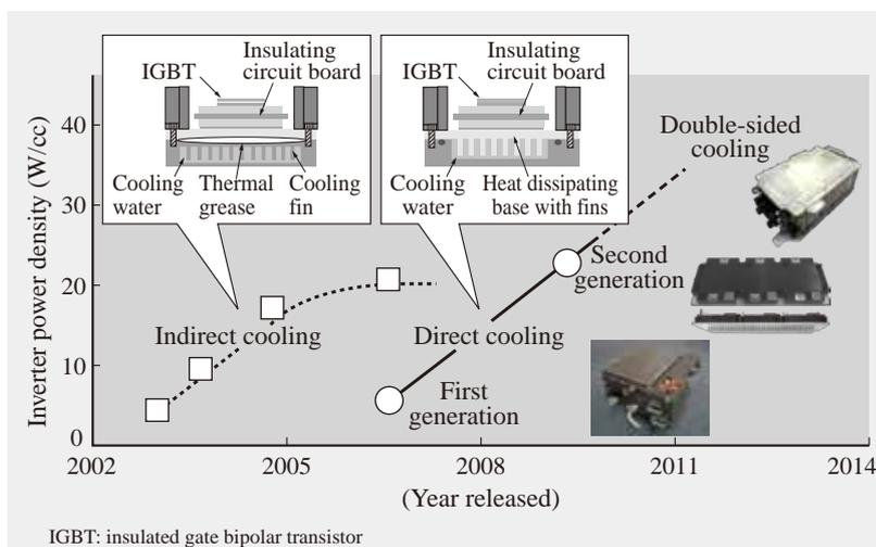
Fig. 2—Ongoing Development of Hitachi Automotive Inverters. The power density has increased year by year. Direct cooling of the power module has been the key to this improvement.
