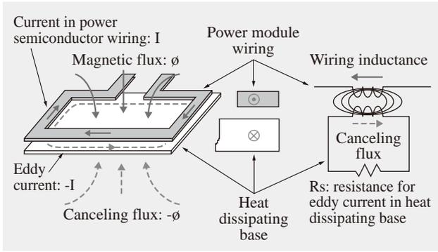
Fig. 3—Technique for Reducing Inductance of Power Module Wiring.
