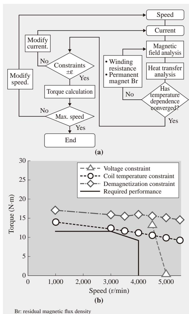
Fig. 6—Flow Chart of Constraint-limited Speed/Torque Characteristics Calculation (a) and Example Calculation of Maximum Torque Possible while Satisfying Constraints (b). The calculation calculates the speed/torque characteristics for the motor based on three constraints (temperature, magnet demagnetization, and voltage).
